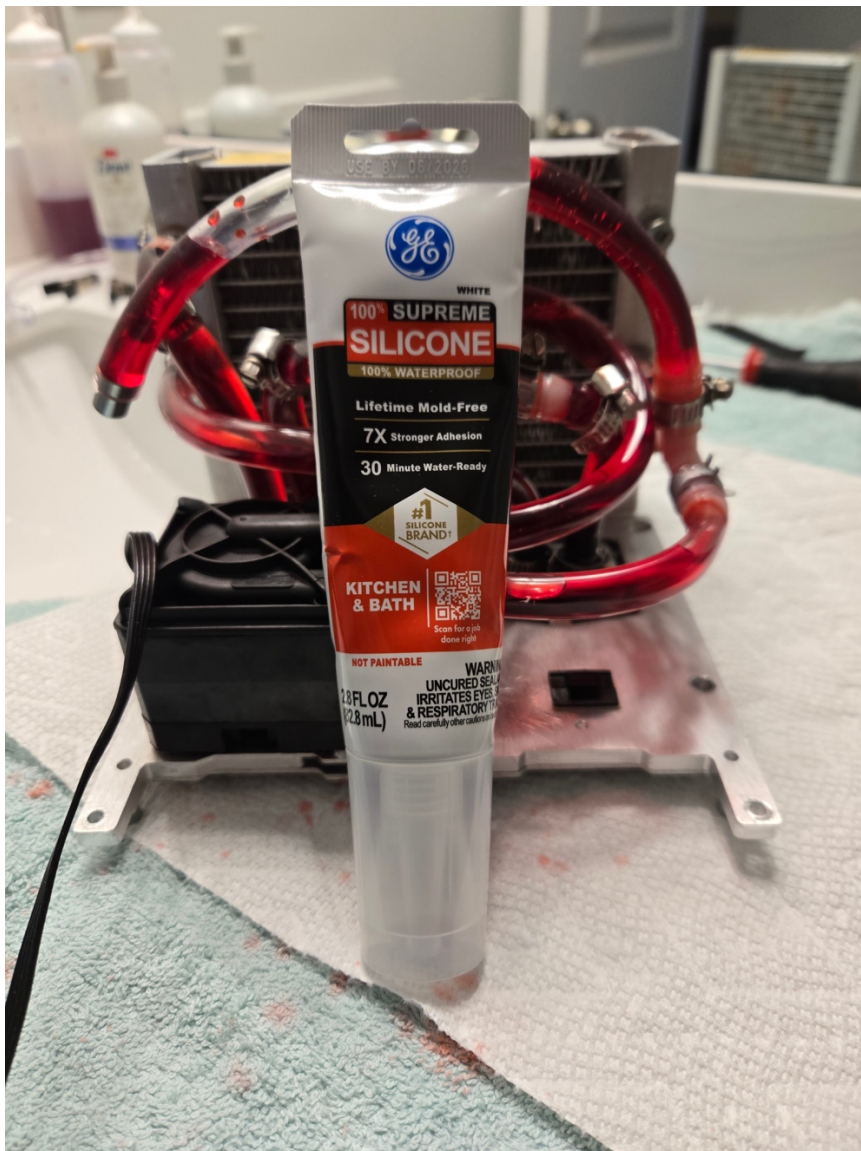
GE Silicone Sealant Used to Seal Pin Prick Holes
