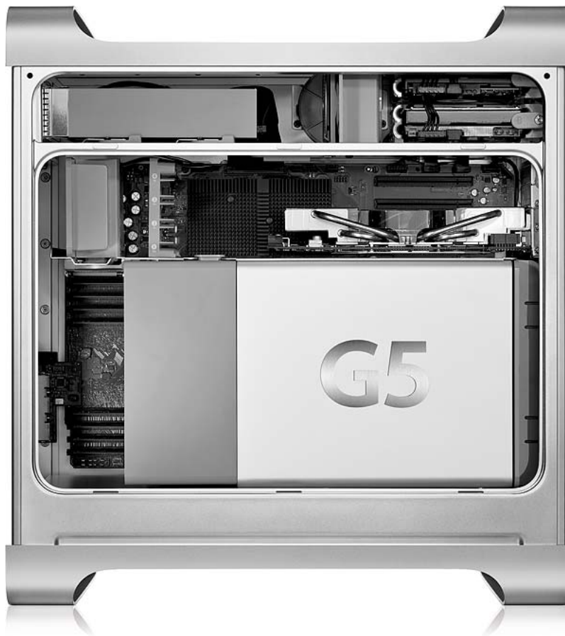
Late 2005 Power Mac G5 Quad Interior
