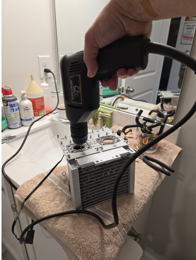
Drilling Out the Screws Holding the Cooling block
